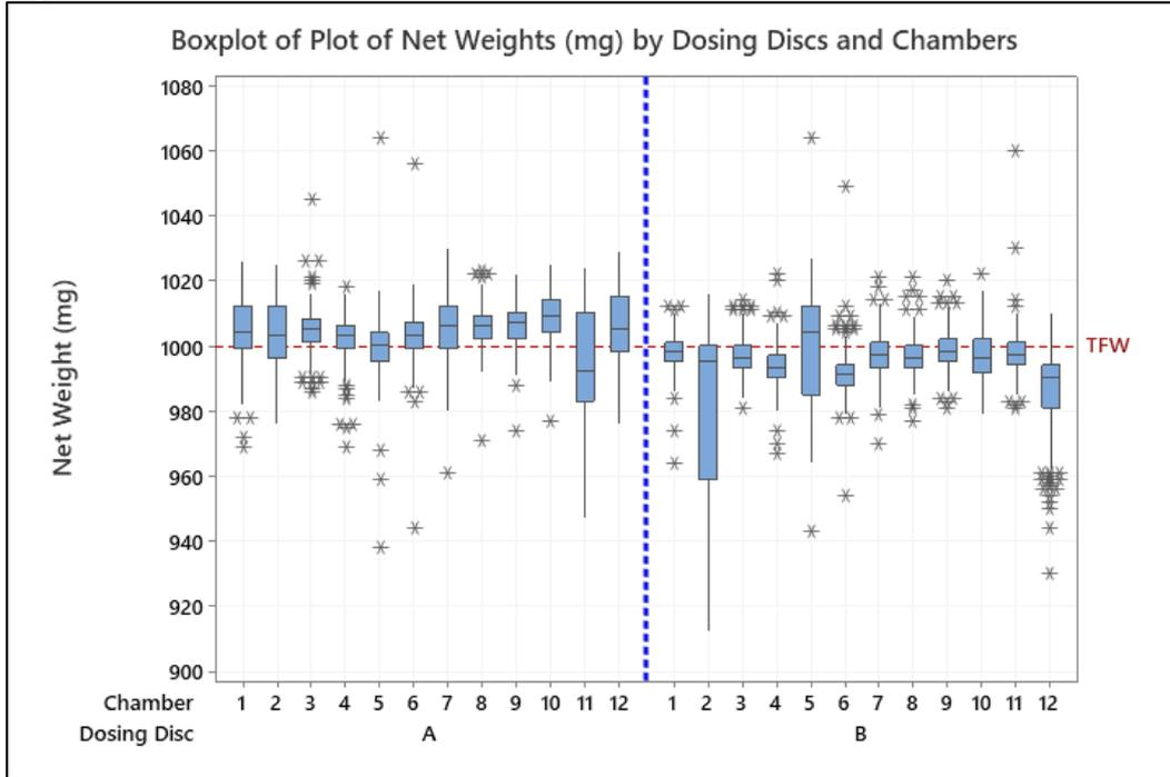
The greater variability associated with chamber 11 of disc A and with chambers 2 and 5 of the disc B is here even more graphically evident (Figure 11).
