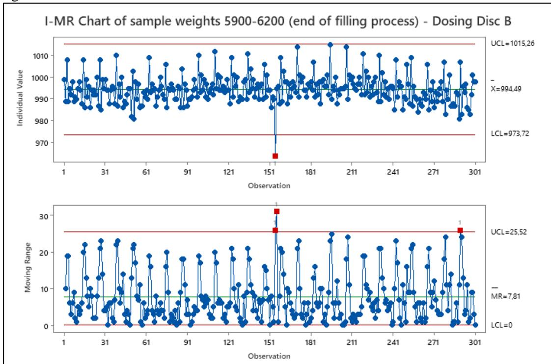
These control charts provide valuable detailed information, but do not account for the difference between the amount of powder dosed on average by the two discs and initially illustrated in Figure 1. To understand this aspect, it is necessary to analyze the behavior of the individual dosing chambers. Figures 8 and 9 show the interval plots of the individual chambers for each dosing disc.
