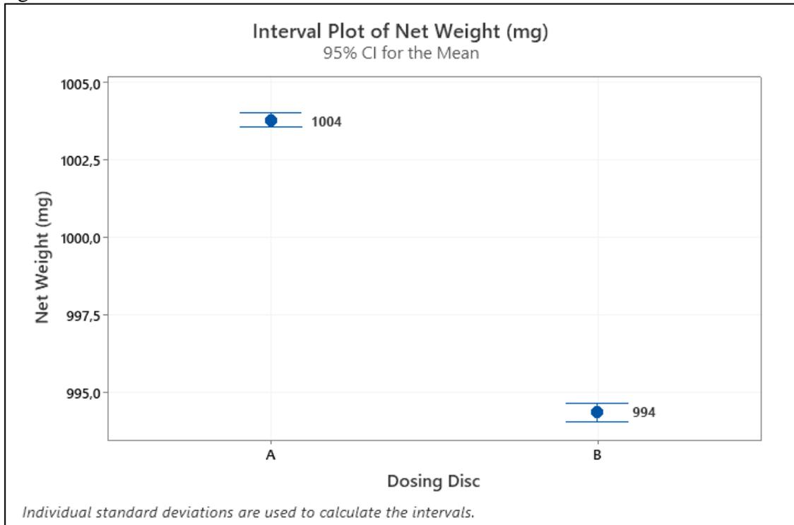
This graph immediately shows a difference of 10 mg, on average, between the quantity dosed by disc A compared to that dosed by disc B.
