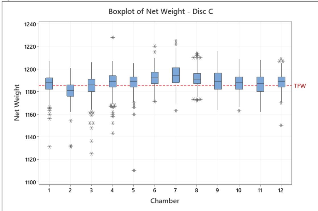
For a more precise comparison between the behaviors of the various chambers in Figure 12, the four box plots relating to the weights delivered by the chambers are shown (Figure 15), while the corresponding histograms are displayed in Figure 16.
