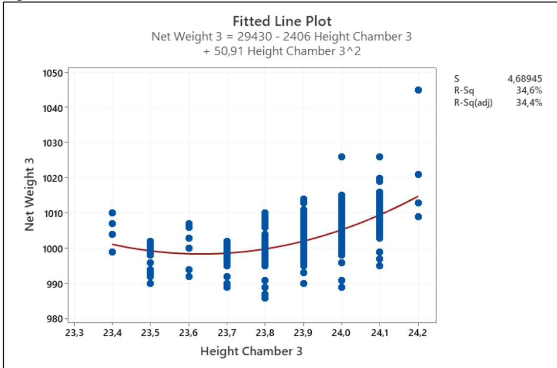
The Analysis of Variance associated with the model, and summarized here below, confirms the statistical significance of the quadratic term as well as the linear one.
