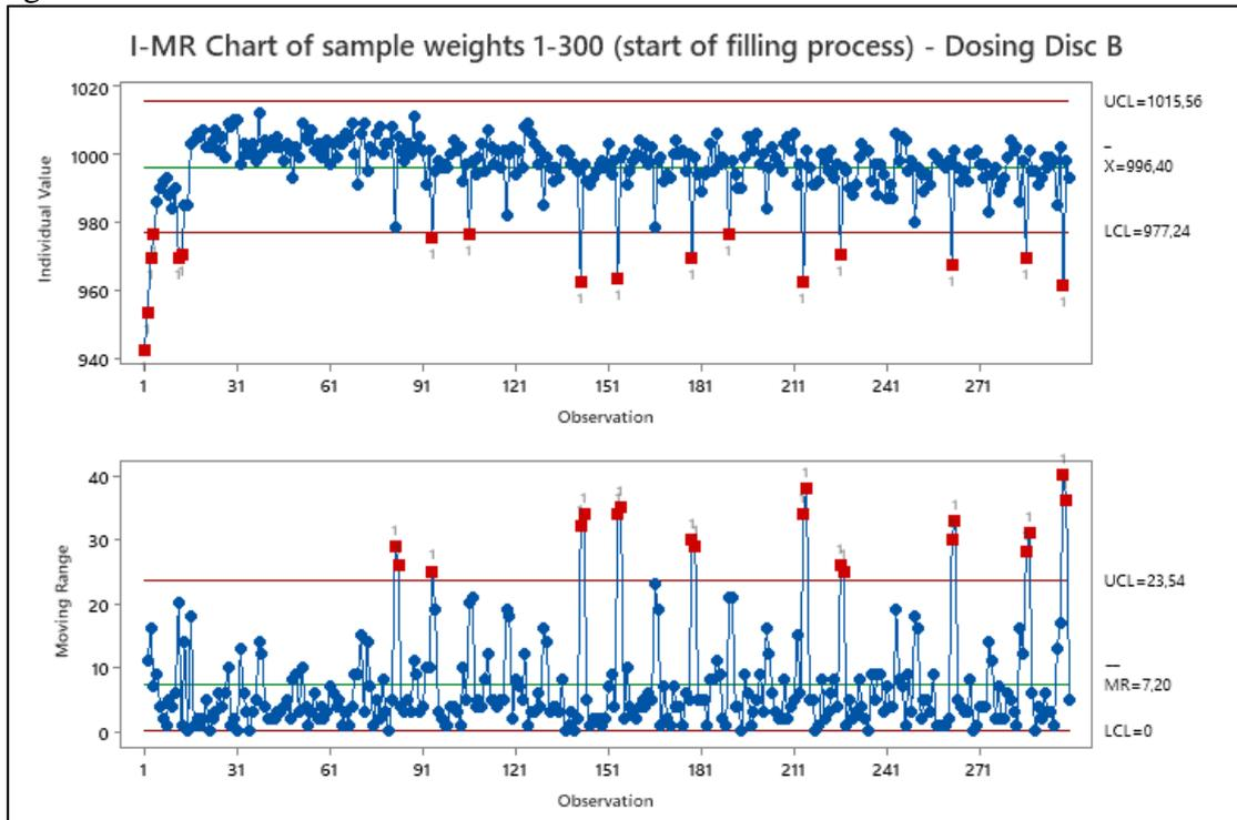
The situation represented above, except for the initial centering phase, appears to be characterized by a greater variability than that observed for the dosing disc A (see Figure 3). Nevertheless, thanks to the self-compensation system, the weights realign themselves obtaining a situation that is practically ideal still in the middle of the filling process (Figure 6) and which remains practically unchanged until the end of the same (Figure 7).
