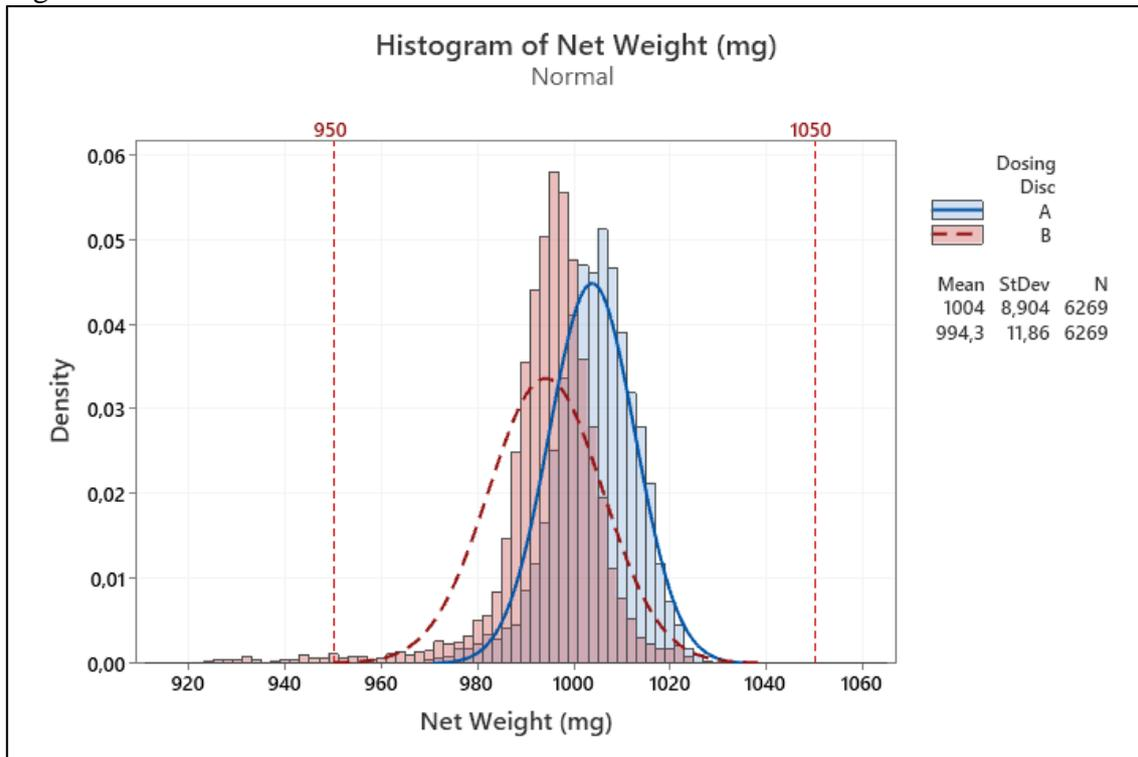
Figure 2 clearly shows that, although both weight distributions tend to be centered around the target value of 1000 mg, the one relating to disc A is less broad. It is in fact characterized by a lower standard deviation with respect to the distribution of the weights delivered by disc B (8.904 vs. 11.86) and is all within  $\pm 5\%$  of the target value (*i.e.*, 950 - 1050 mg).
