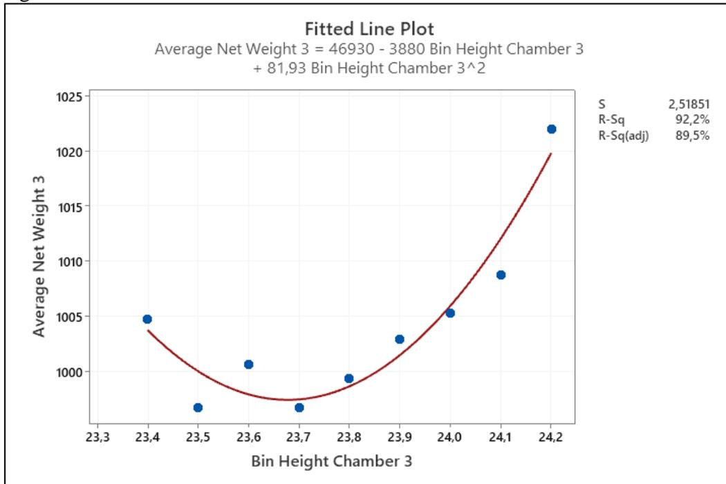
In this last case, the analysis of variance associated with the model shown above indicates the quadratic term as the most relevant.
