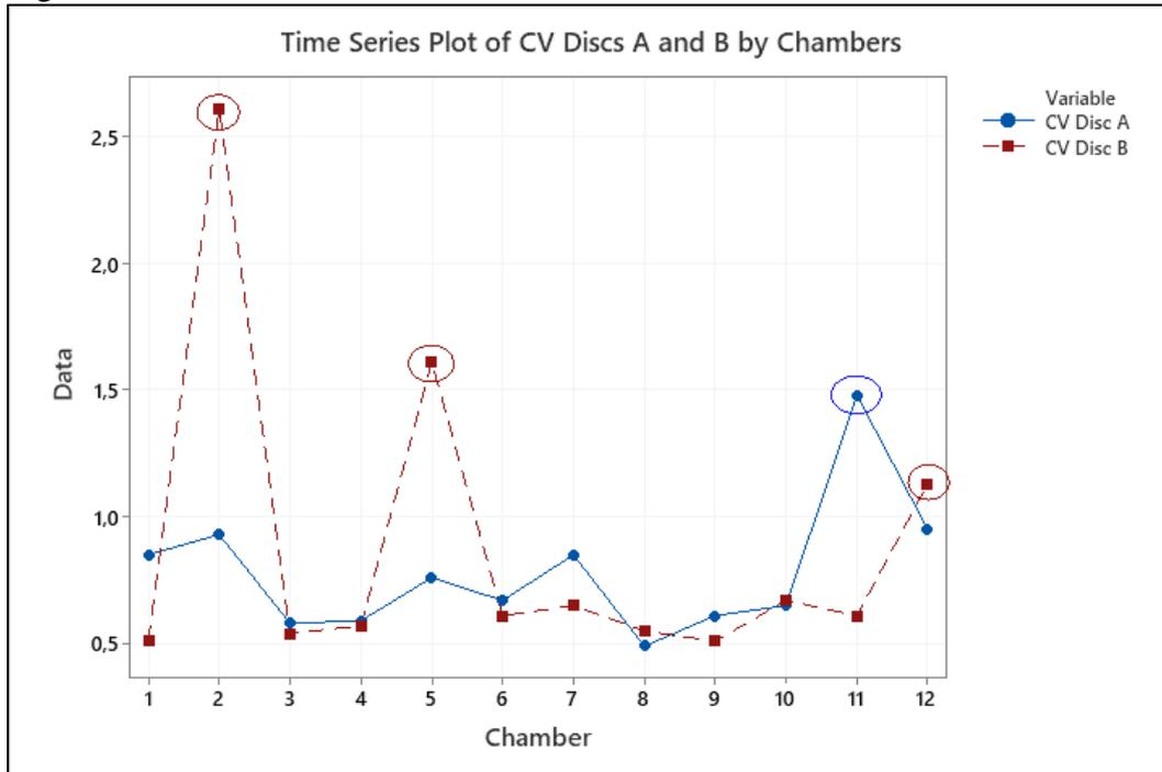
Figure 28 immediately shows the chambers affected by anomalous variability, namely 11 for dosing disc A and 2, 5, 12 for disc B.
